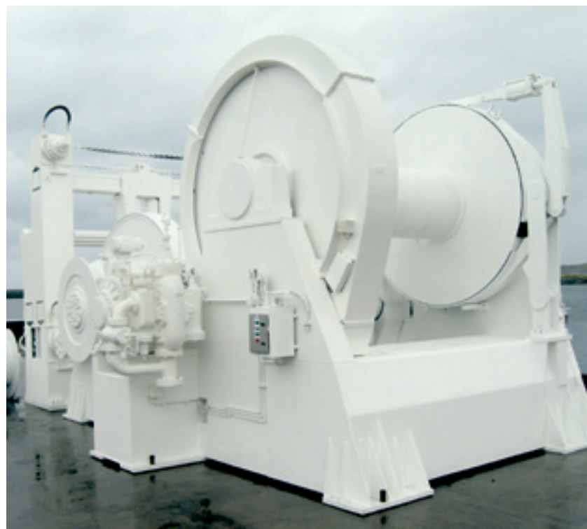
Anchor handling winches work under extreme loads
