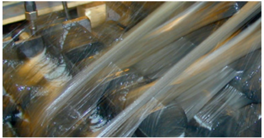
The long-fibred, homogeneous texture of the adhesive lubricant causes a stretching effect, ensuring reliable lubrication also with long intervals
